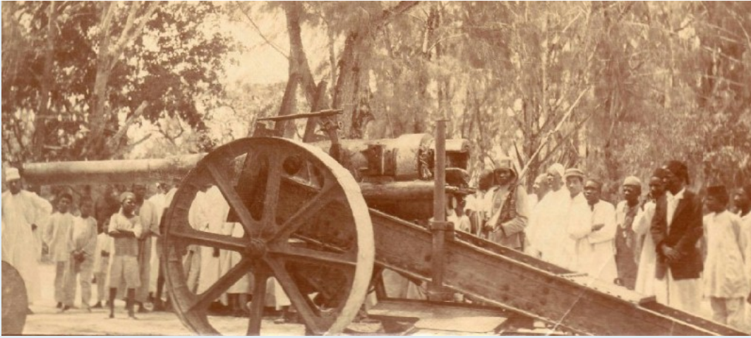
Here is the gun shown shortly after its capture in Bagamoyo. Note the Krupp gun carriage sitting above the axle, its gunners platform, ammunition hoist bar, partial shield and Krupp wheels with eight struts. In the background is an Askari of the British Kings African Rifles standing guard. This photograph was in the collection of Able Seaman William Thomas Clegg RN who served on the HMS Vengeance in East Africa during the First World War, and has kindly been shared with us by his grandson, Bob William Green.
