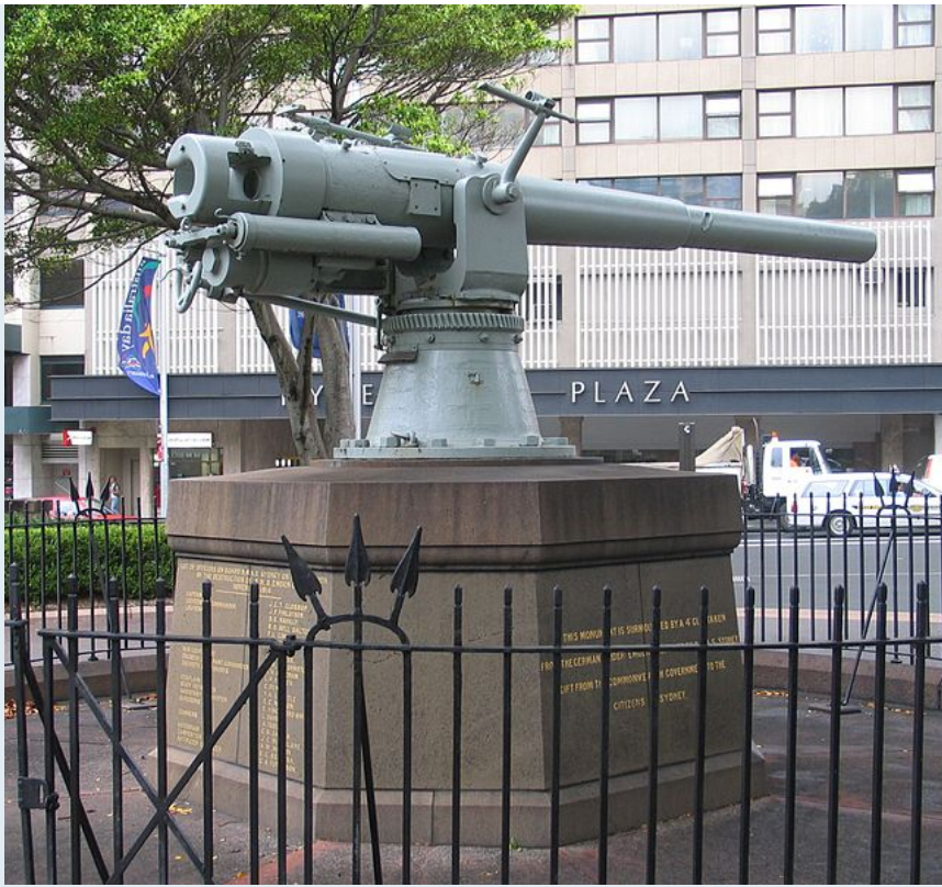
This Emden 10.5cm gun has no flange and was therefore not turret mounted.
